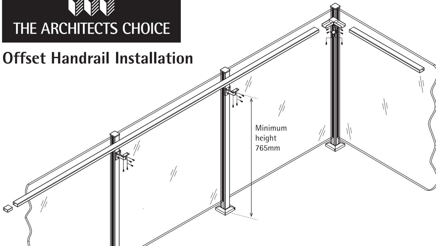
If you have corner joints start by fitting these, this will make it easier to measure straight lengths.
