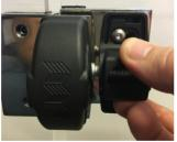
Using a hex key, loosen the screws and adjust the latch body so the latch can close. Remember not to exceed the 10mm gate to panel/post/wall gap.
